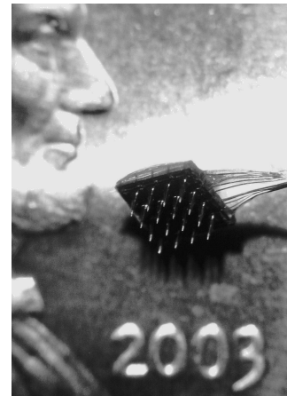
Figure 2: The 4-by-4 version of the Utah Electrode Array, photographed on a penny for scale, was implanted in the feline skull.
