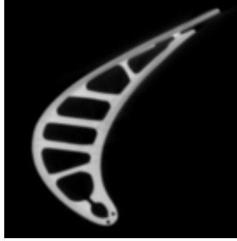
Figure 6.4: Cross-section of blade showing struts
