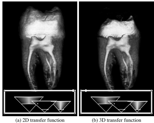
Figure 2: In (a), the 2D transfer function is intended to render all material interfaces except the enamel-background boundary at the top of the tooth. However, by using a 3D transfer function (b), with lower opacity for non-zero second derivatives, the previously hidden dentin-enamel boundary is revealed.
